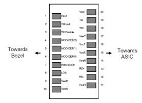
**SFP Transceiver Electric Pad Layout**
