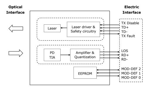
The transceiver is fundamentally consisted by two parts: transmitter and receiver. The transmitter features a TTL logic level Disable signal and a Fault indicator. The receiver features a TTL logic Loss of Signal (LOS) detection. For the access of serial identification information, an EEPORM is used to store the required data via the 2-wire serial CMOS EEPROM protocol. The detailed signal descriptions are listed in the following sections.
