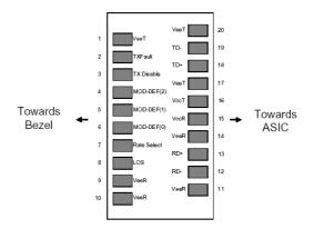
**SFP Transceiver Electric Pad Layout**
